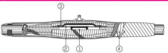
This product is a combination of a Cold-Shrink insulating body encapsulated in an injected resin outer protection.
